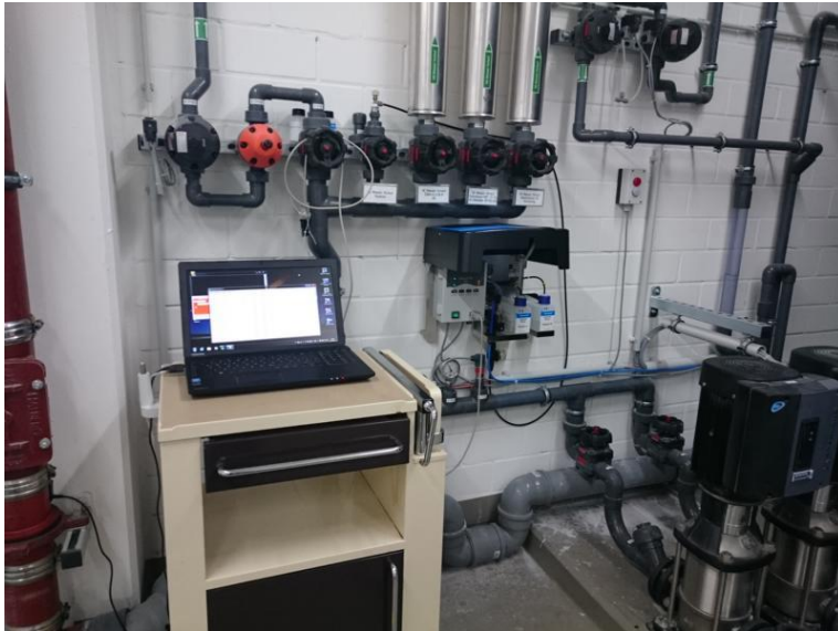
Measurement value logging during the practical testing of the Testomat® 808 SiO 2
