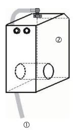
➤ If water sprays from the tube ① of the measuring chamber ②, reduce the amount of inlet water via the manually operated shut-off valve. It should take 2 to 6 seconds to fill the measuring chamber!
