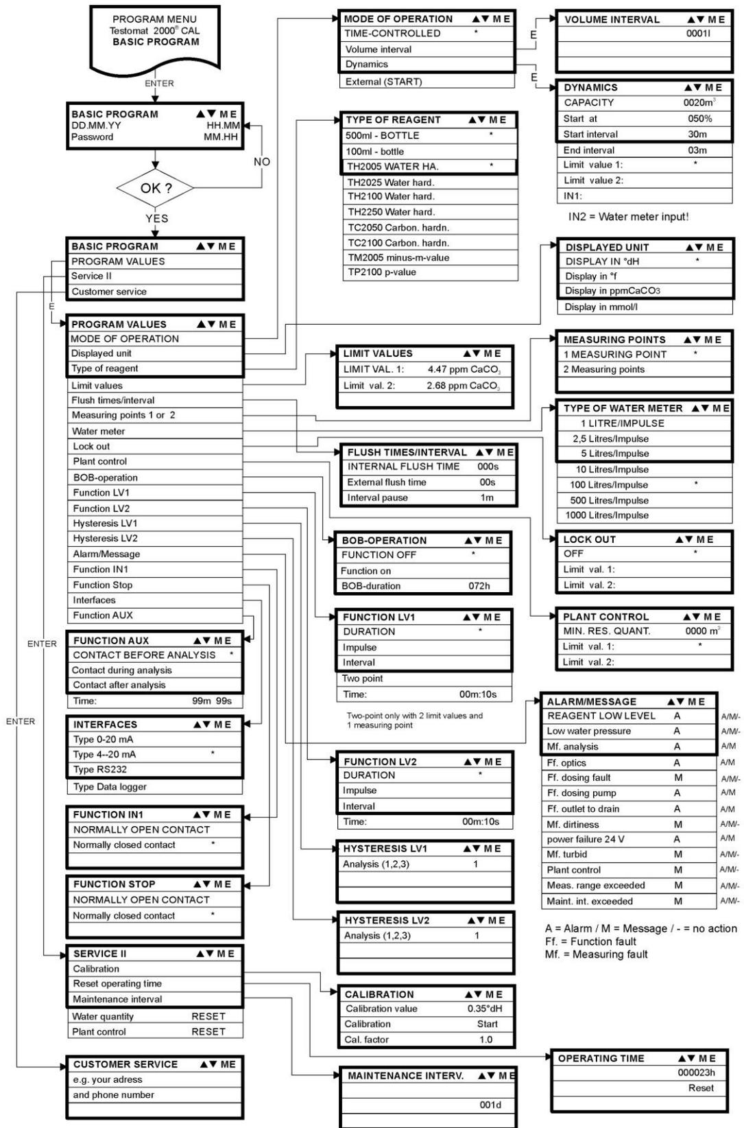
Call the basic factory program by simultaneously pressing and holding down the "M" and "i" keys while switching on the instrument. CAUTION, the last set of programming will be erased!
