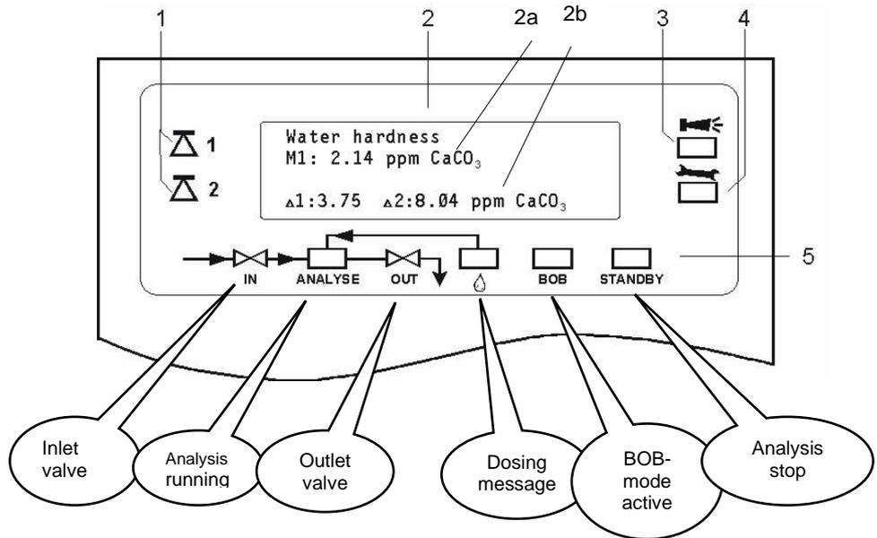
All error and warning messages are alternately shown in line 1 of the standard display!
