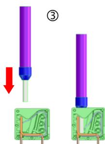
Insert the conductor with ferrule or the solid conductor into the round input.
