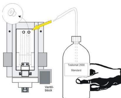
The filling level falls to the intended sample volume. The measured value is determined and the correction value is calculated. The factor is shown on the display.
