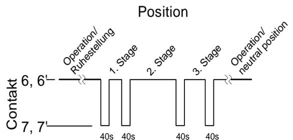
For versions with an impulse switch control, the output switches for 40 seconds at the beginning of each stage (terminal 7 or 7').
