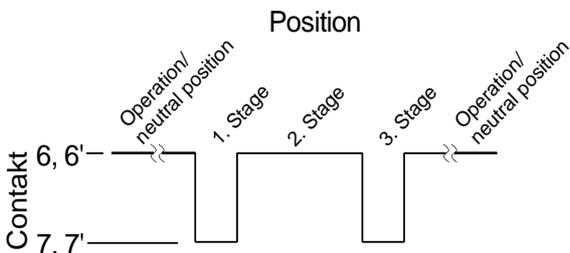
For versions with a change-over contact control, the output changes after each regeneration stage. With an odd number of the mechanical positions, operating position reset has to occur via the synchronous contact (operating switch).
