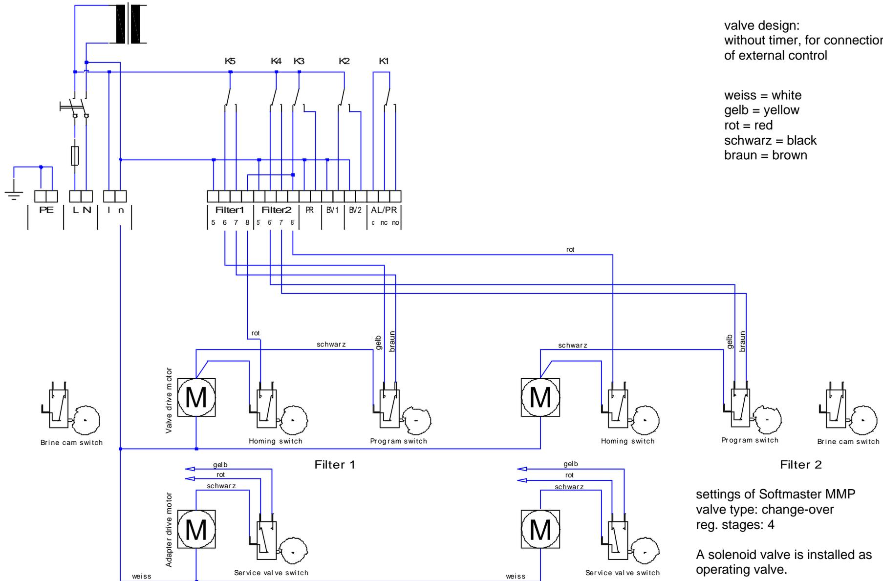
**Connection example for control valve Fleck9000 (single-filter plant)**
