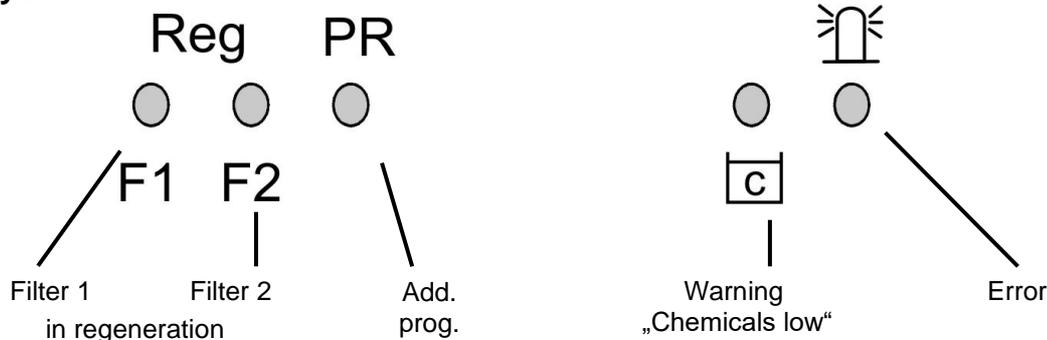
The displays signal operating statuses, plant functions and current error messages:
