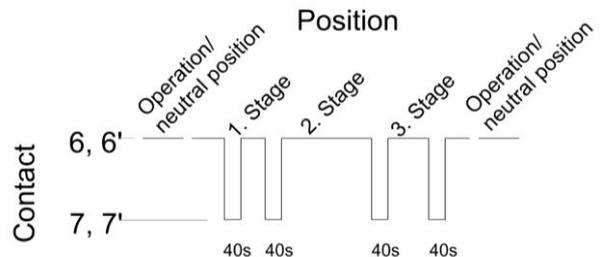
For versions with an impulse switch control, the output switches for 40 seconds at the beginning of each stage (terminal 7 or 7').
