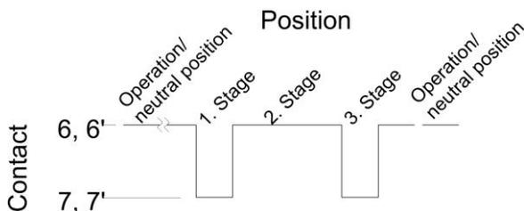
For versions with a change-over switch the output changes after each regeneration stage. With an odd number of the mechanical positions, operating position
