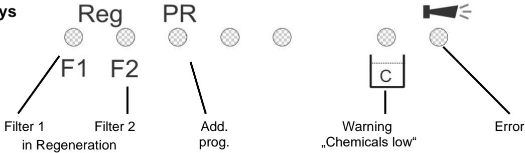
The displays signal operating statuses, plant functions and current error messages:
