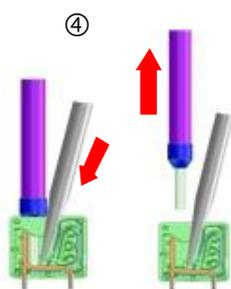
1. Insert a screwdriver into the square opening without force in order to open the terminal.
