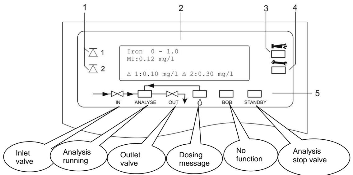
All error and warning messages are alternately shown in line 1 of the standard display!
