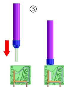
Insert the conductor with ferrule or the solid conductor into the round cable input.
