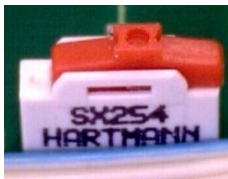
Switch position right (delivery status)
