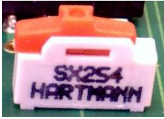
Switch position left (delivery status)
