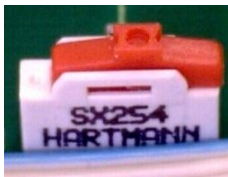
Switch position right (delivery status)
