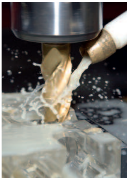
Milling of a BOB measuring chamber block
