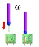
Insert the conductor with ferrule or the solid conductor into the round input.
