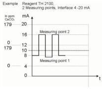
The range of the current interface is divided. The range 4 - 12 mA is available for the measured value from measuring point 1 and range 12 - 20 mA for the measured value from measuring point 2.
