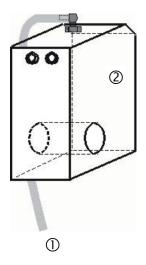
➤ If water sprays from the vent hole ① of the measuring chamber ②, reduce the amount of inlet water via the manually operated shut-off valve. It should take 2 to 6 seconds to fill the measuring chamber!
