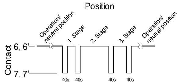
In the case of impulse switches, the output switches for 40 seconds at the beginning of each stage (terminal 7 or 7').
