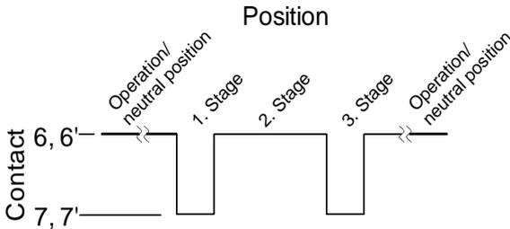
In the case of change-over switches, the output changes after each regeneration stage. If the number of mechanical positions is odd, the return movement to
