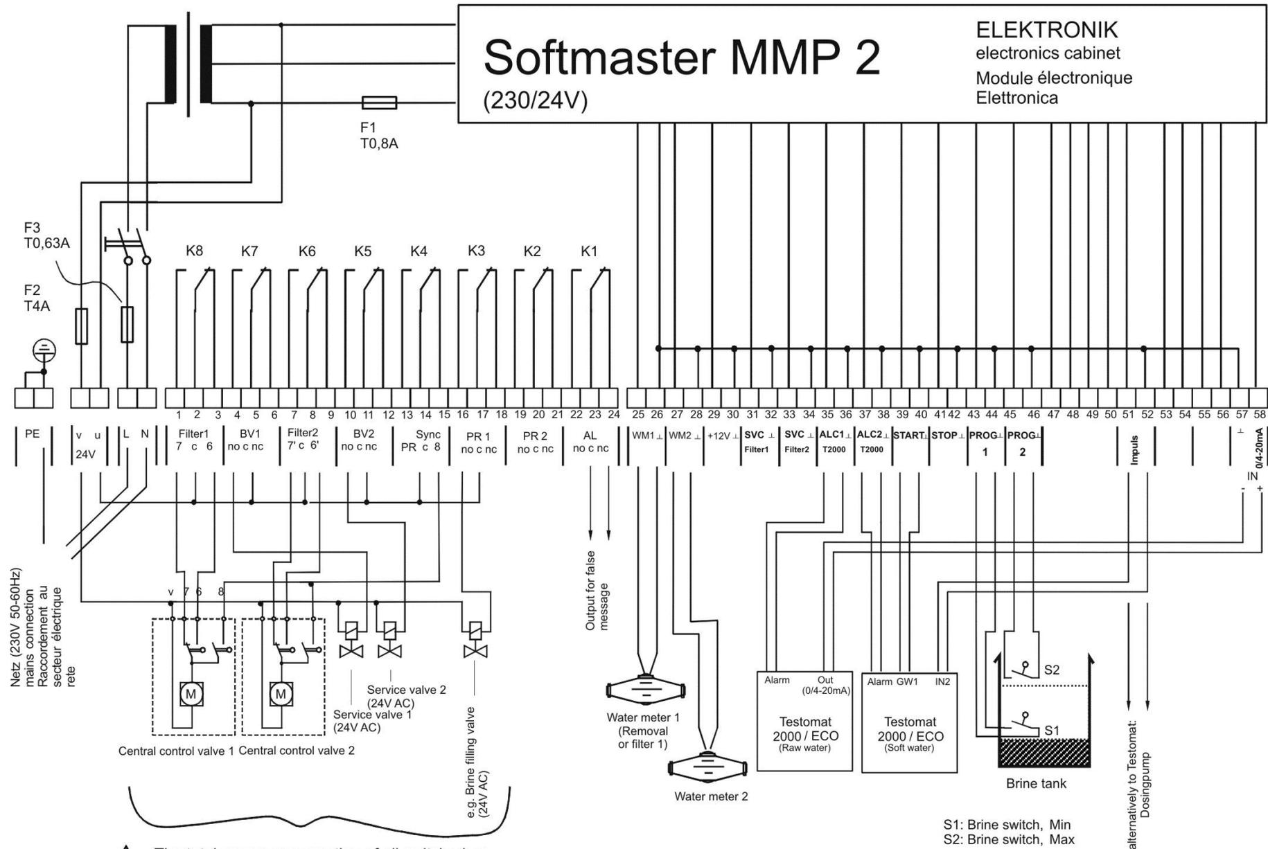
**!** The total power consumption of all switched-on components should not exceed 90 VA!
