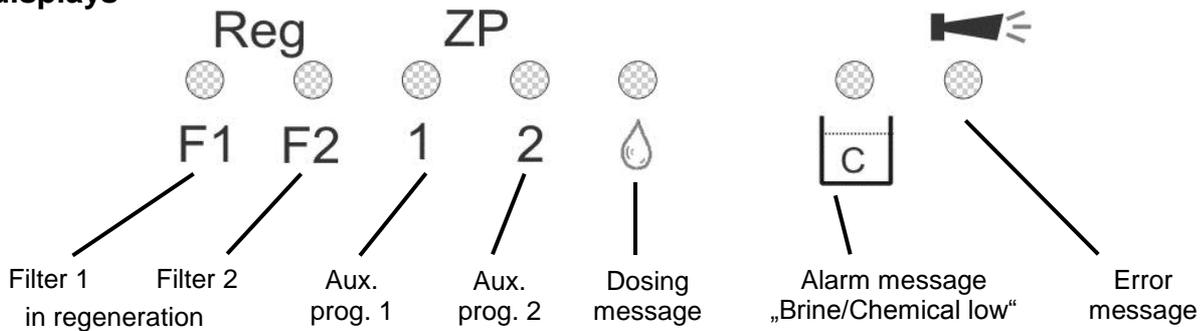
The LEDs display operating statuses, plant functions and pending error messages:
